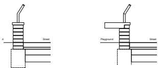
Sketch sections through typical wall and wall/seat.
